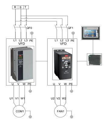
VFD compressor / VFD fan control
