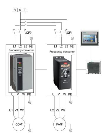
The most prominent feature of a variable frequency speed drive chiller is the frequency converter that is added to drive the compressor; its starting current is 60% lower than that of the driver of a traditional unit. In addition to compressor control, convertible frequency technology can also be use to control fans, and water pumps among others.
