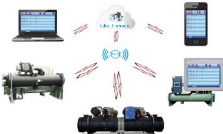
Central A/C cloud service system
